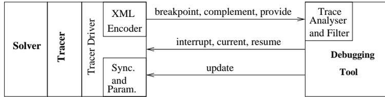
Figure 8.1: Tool/Tracer Architecture and Command Schemata
