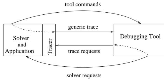
Figure 1.2: Communications between Solver and Debugging Tool
